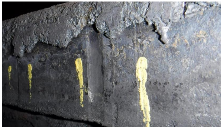
Figure 2: Indentation marks on a slab of a defective roll.
